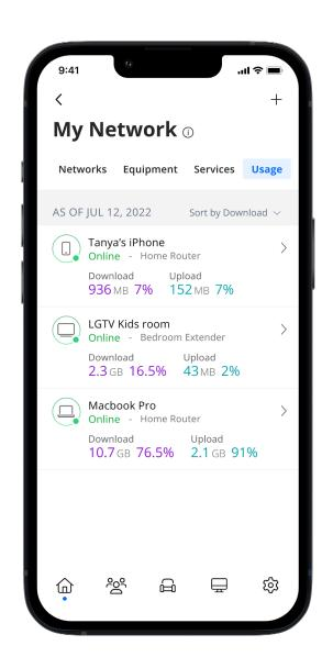
Network Usage is organized by device. From this view, you can see basic information about usage from each Wi-Fi connected device on your network, including: 1. Device identification and whether the device is connected to Wi-Fi 2. What network device it is connected to 3. Network usage 4. The amount of data that has been used by this device Network usage is updated each time you run a bandwidth test through the app. Note: This feature is only available with a GigaSpire BLAST.
