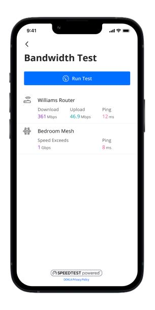
The easiest way to run a bandwidth test is by tapping into "My Network" and then "Bandwidth Test" icon. Then simply tap the Run Test button. The speed test will first run between the GigaSpire BLAST and the Internet and then will conduct a speed test between any mesh units and the GigaSpire BLAST. Results will show as a notification and update at this location. Note: This feature is only available with a GigaSpire BLAST.
